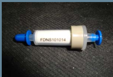
Photo 2: new 2mL cartridge design for DGA,N resin with grey color code ring.
