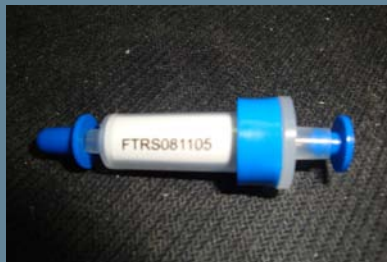
Photo 1: new 2mL cartridge design for TRU resin with blue color code ring.
