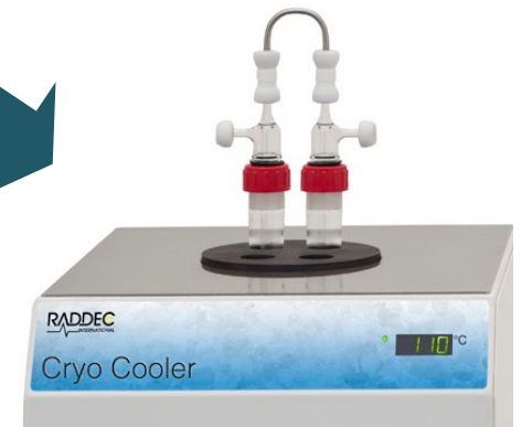
Combustion water recovered under vacuum
